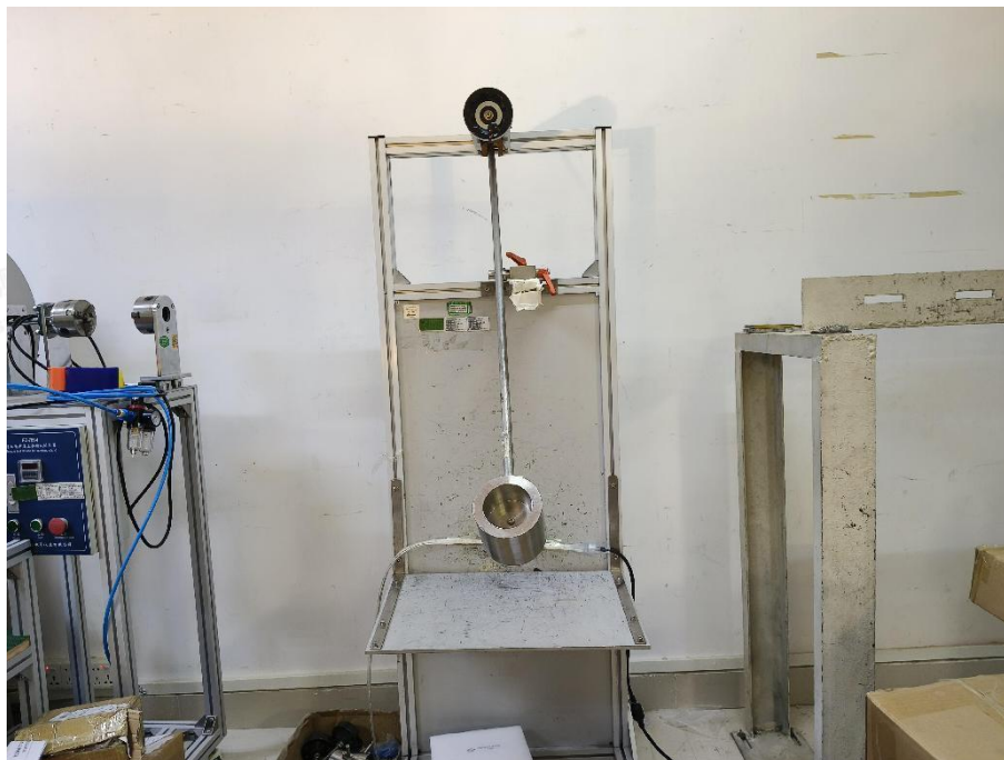
Photo 3: IK10 test of model 2835-180-230V-XXX
