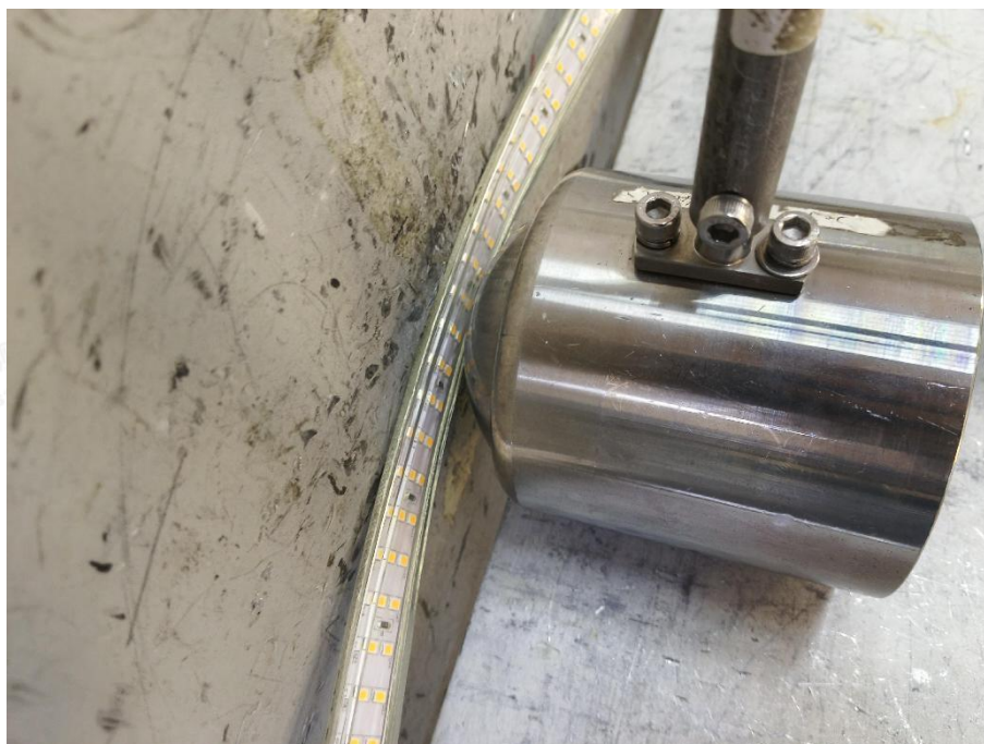
Photo 4: IK10 test of model 2835-180-230V-XXX
